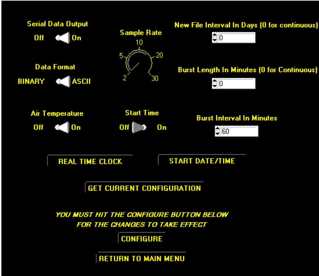
The configuration control panel is shown above. From this it is possible to configure a wide range of features. To start, press the GET CURRENT CONFIGURATION button and the dials and indicators will change to reflect the current settings of the instrument. Please see the detailed data sheet for the Wave Logger III to understand the function of the various features.
